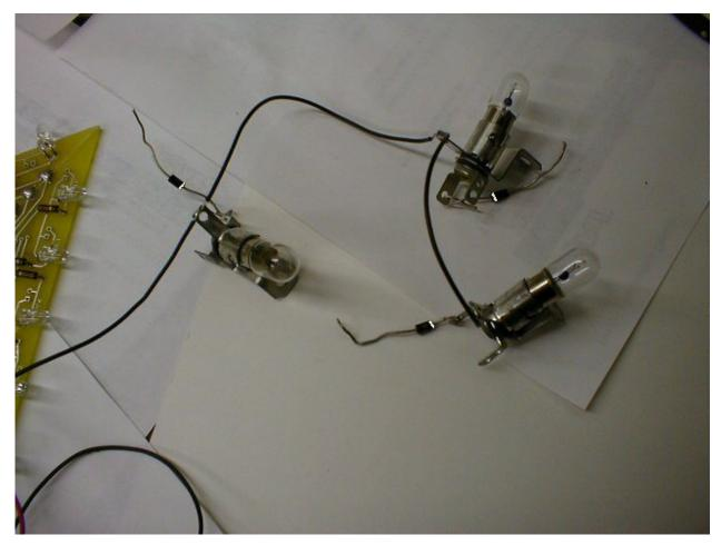
There are three more red wires that we need to connect before we can say we are done with the brain. Connect one of these wires to each bulb on the DIODE side and then shrink wrap the solder joint. The order you connect them is not important, just one wire per bulb diode and you will be fine.
