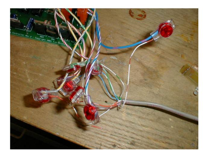
Power for this setup is +12vdc. The Red and Black is your power feed to the controller, Red is +, black is -.
